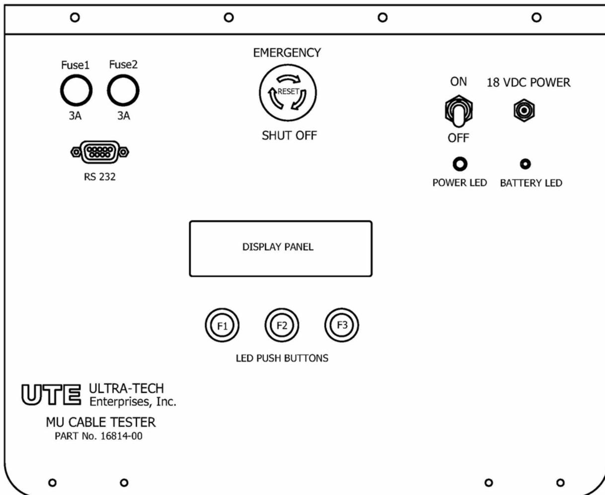
**Power On / Off Switch** – Controls the main power to the MU Tester Unit. Power is supplied from the AC to DC power adapter or from the internal battery.
